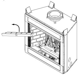
Figure 13 - Removing Front Refractory Access Panel
